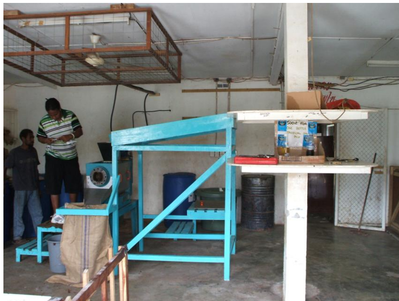
Screw press used to expel the Tamanu Oil
