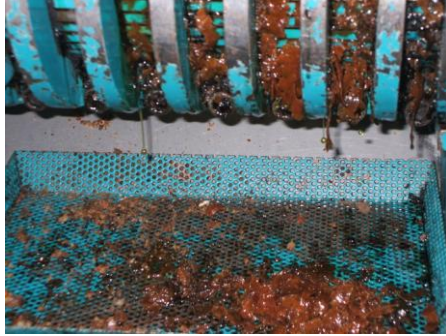
Tamanu Oil being cold pressed
